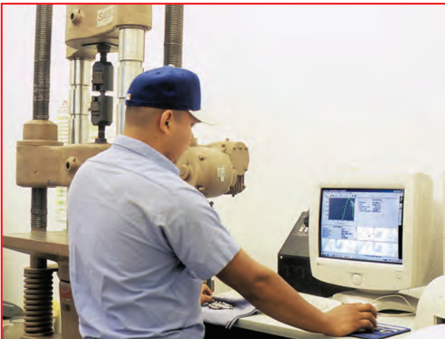
A computer-controlled Instron tensile machine is used to determine the ultimate tensile strength of studs and bolts.
