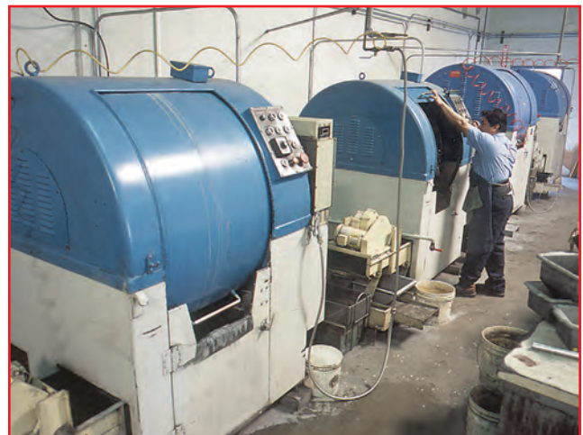
ARP's popular stainless steel engine & accessory fasteners are polished to a brilliant luster using this specialized equipment.
