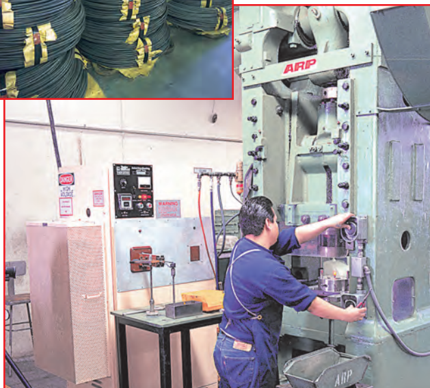
Material comes from the mill in large coils...which subsequently will be fed into cold-headers and formed into bolts.
