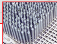
ARP performs the thread rolling operation after heat-treating, which results in a fatigue strength up to 10-times higher than fasteners with threads rolled prior to elevating the material's tensile strength.
