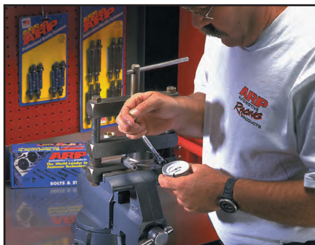
A rod bolt stretch gauge is one of the most important tools a serious engine builder can own. It's valuable in properly setting up a rod for resizing, obtaining the proper torque load when installed in the engine, and monitoring the condition of the bolt while in use.
