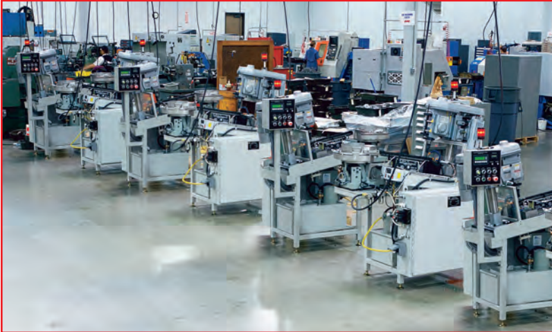
A series of CNC-threading machines are employed by ARP to accurately tap the threads in nuts. Tolerances held are 5 times better than aerospace standards.
