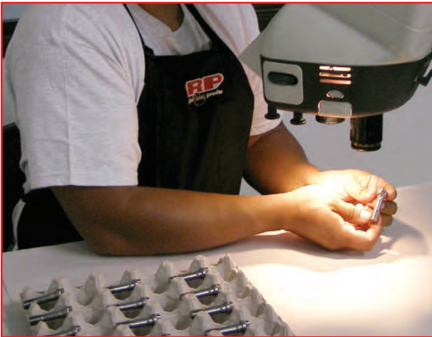
High powered magnifiers are used to carefully inspect critical components. ARP's quality control team is relentless!
