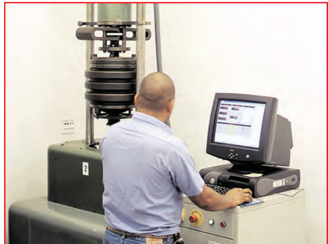
ARP has two of these highly sophisticated Amsler fatigue machines, which check fasteners through millions of cycles.
