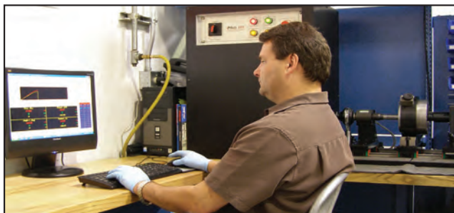
ARP's computer-controlled torque-tension machine can apply a given "torque" or "angle" to a fastener and measure the actual preload. Through test cycles, it is possible to chart the "preload scatter" with various fasteners and lubricants.
