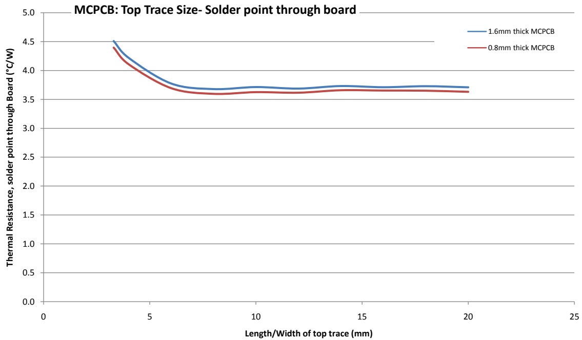
Chart 2: Thermal resistance for MCPCB with varying thermal pad size
