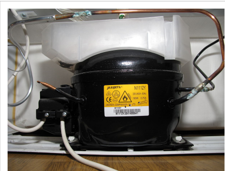
A small hermetically sealed compressor in a common consumer refrigerator or freezer; it typically has a rounded steel outer shell that is permanently welded shut, and which seals operating gases inside the system. There is no route for gases to leak, such as around motor shaft seals. On this model, the plastic top section is part of an auto-defrost system which uses motor heat to evaporate the water.
