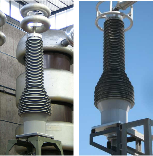
Fig. 8: 245 kV dry self supporting outdoor termination during PQ test.
