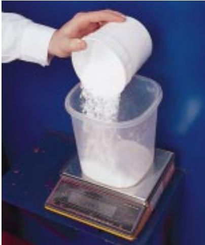
Weighing the polyolefin powder
