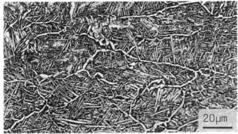
Fig. 35: Necklace microstructure, "beta-deformed" condition, LM.
