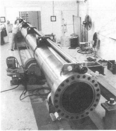
Fig. 81: Photos of heavy walled tubular drilling riser for a high pressure petroleum well (courtesy RMI Corp.).
