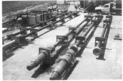
Fig. 77: Photo of Ti-6Al-4V taper stress joints used in an off-shore oil platform (courtesy RMI Corp.).
