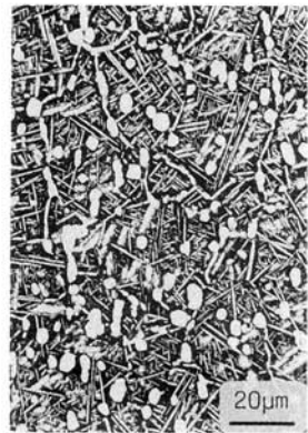
Fig. 30: Bi-modal microstructure, LM.
