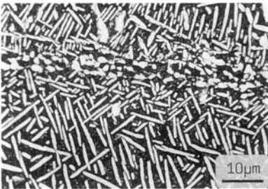
Fig. 34: Necklace microstructure, "through-transus" processing.
