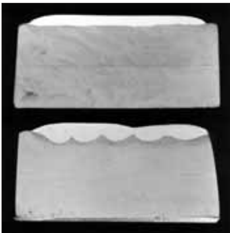
Figure 4.16. Weld bead shape – strip versus wire
