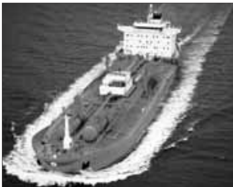
Figure 1.11. Chemical tanker – tanks in 2205 stainless steel
