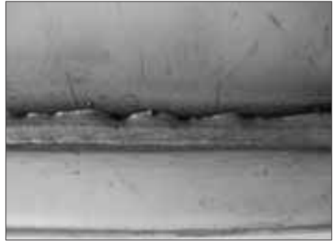
Figure 5.1. Lack of fusion – MIG
