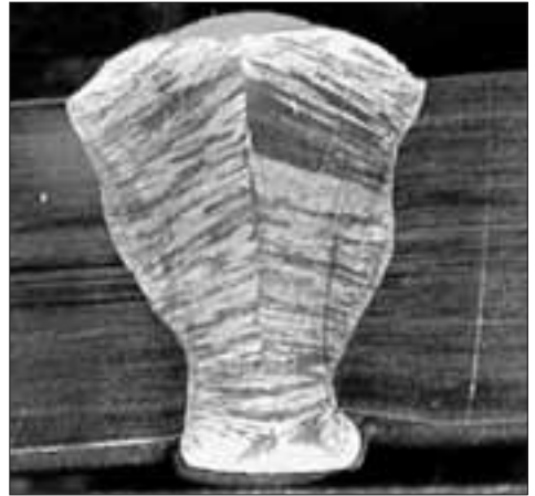
Figure 5.12. Excessive weld metal – MIG 316L-Si
