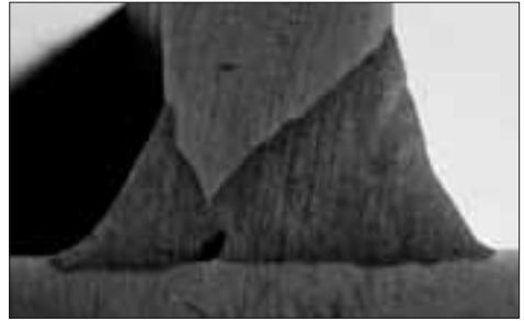
Figure 5.6. Slag inclusion in a 2205 FCA weld
