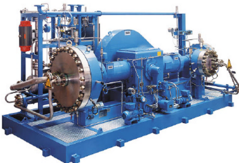
Picture 16: Type: Diaphragm Compressor MKZ800-5/470-10/315-25 No. of rev.: 360 rpm Stages: 3 Medium: high purity Hydrogen Suction press.: 5 bar abs Disch. press.: 201 bar abs Capacity: 250 m 3 /h (VN) Motor power: 68 kW Execution: ready for operation
