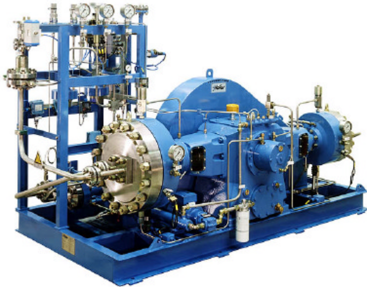
Picture 14: Type: Diaphragm Compressor MKZ450-10/280-25 No. of rev.: 460 rpm Stages: 2 Medium: high purity Hydrogen Suction press.: 10-14 bar abs Disch. press.: 251 bar abs Capacity: 142 m 3 /h (VN) Motor power: 33 kW Execution: ready for operation
