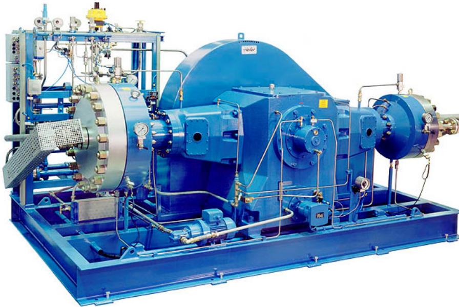
Picture 19: Type: Diaphragm Compressor MKZ680-10/450-40 No. of rev.: 360 rpm Stages: 2 Medium: Hydrogen Suction press.: 18 bar abs Disch. press: 281 bar abs Capacity: 580 m 3 /h (VN) Motor power: 135 kW Execution: ready for operation
