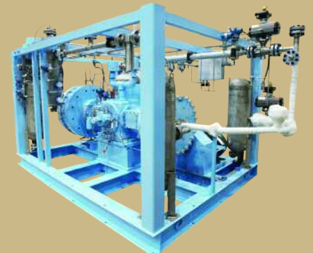
PDC-5-100-350. 40 hp motor, 40" & 29" diameter heads, Vinyl Fluoride service, 100% radio graphed welded piping, Plant application.
