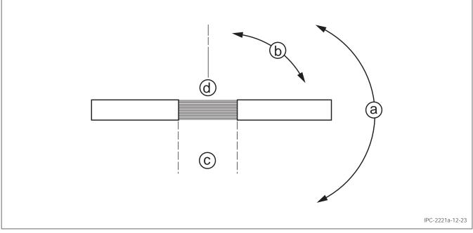
Figure 12-23 Bending Test
