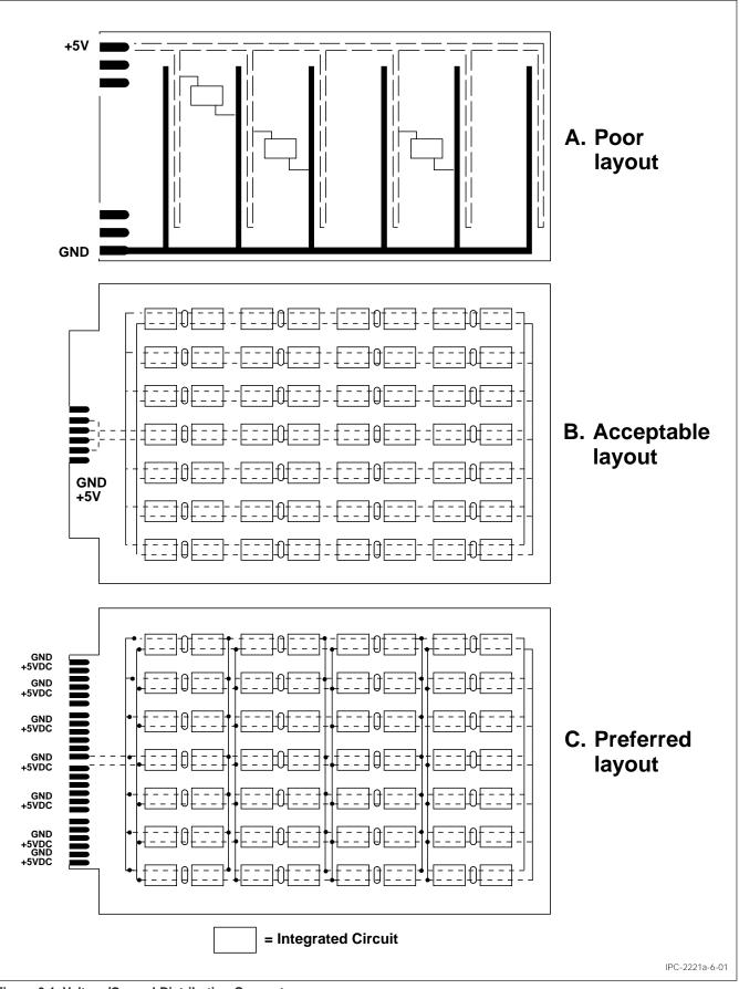
Figure 6-1 Voltage/Ground Distribution Concepts
