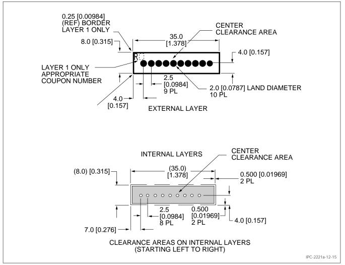
Figure 12-15 Test Coupon R, mm [in]
