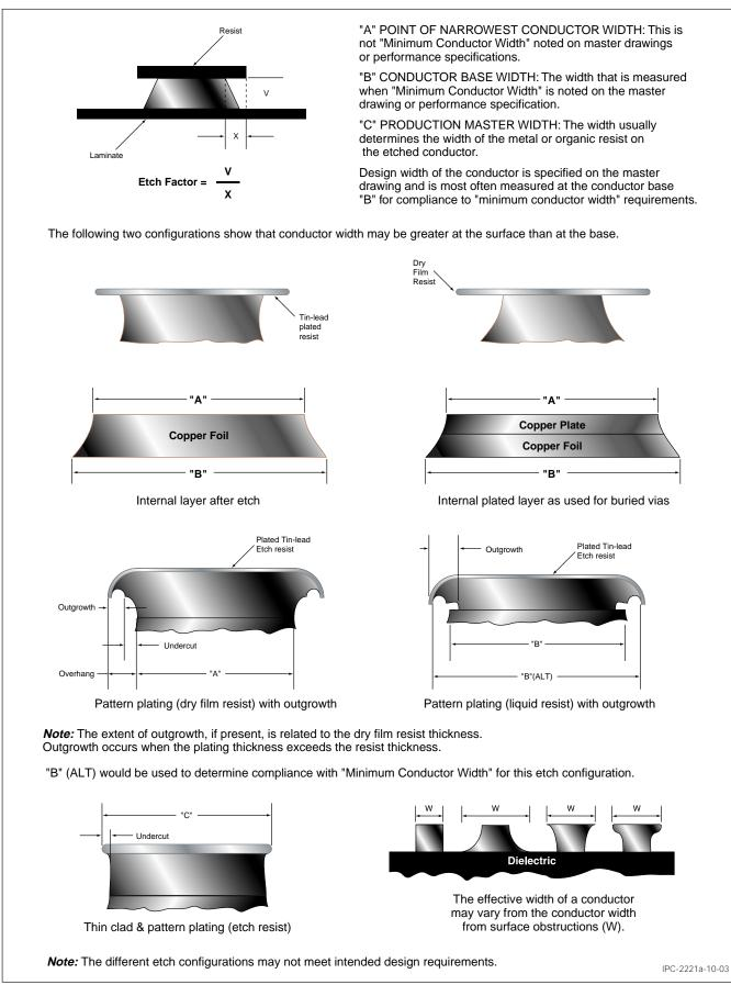
Figure 10-3 Etched Conductor Characteristics
