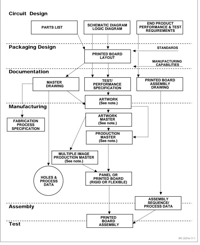
Note: The term "original" may be used to preface any of the drafting and photographic tooling terms used in the figure. The "original" is not usually used in manufacturing processes. In the event a "copy" is made, the copy **shall** be of sufficient accuracy to meet its intended purpose if it is to take on the name of any one of the terms used in this figure. Other adjectives may also be used to help describe the kind of copy, e.g.: "nonstable," "first generation," "record," etc.
