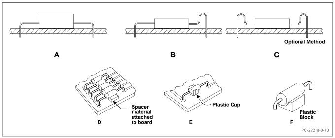
Figure 8-10 Typical Lead Configurations
