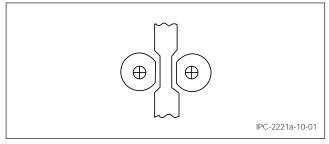
Figure 10-1 Example of Conductor Beef-Up or Neck-Down
