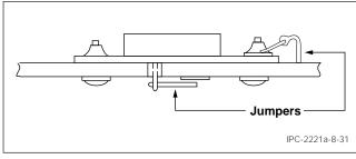
Figure 8-31 Metal Power Package with Noncompliant Leads
