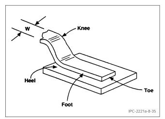
Figure 8-35 Heel Mounting Requirements
