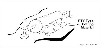
Figure 8-6 Adhesive-Bonded Axial-Leaded Component
