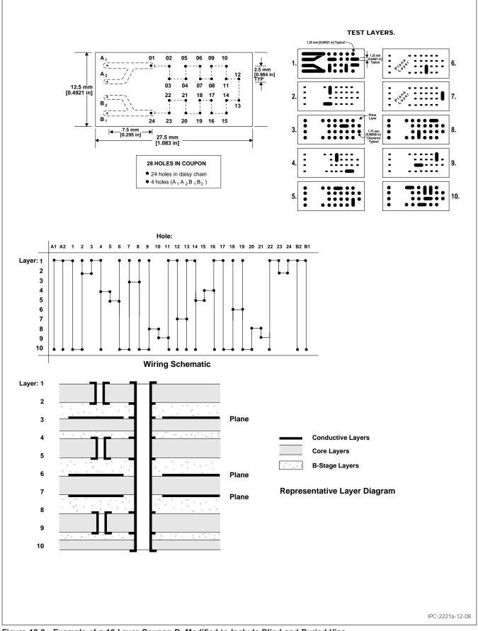
Figure 12-8 Example of a 10 Layer Coupon D, Modified to Include Blind and Buried Vias
