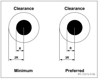
Figure 5-6 Fiducial Clearance Requirements
