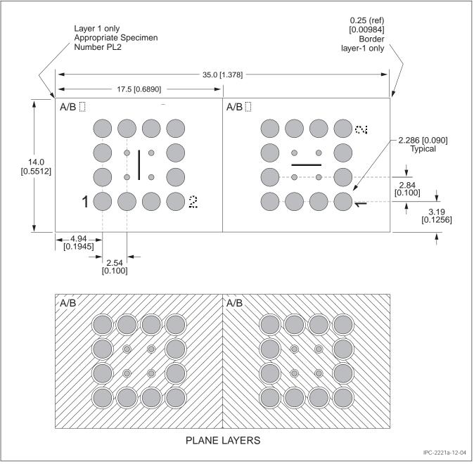
Figure 12-4 Test Coupon A/B, mm [in]
