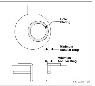
Figure 9-3 Internal Annular Ring
