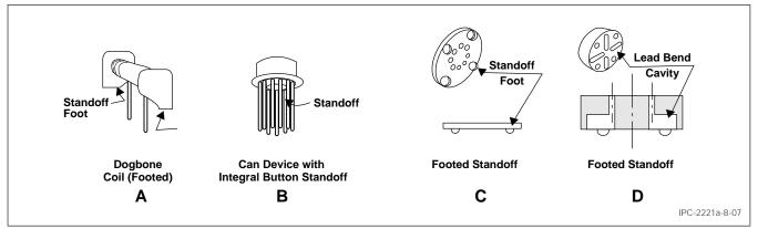
Figure 8-7 Mounting with Feet or Standoffs
