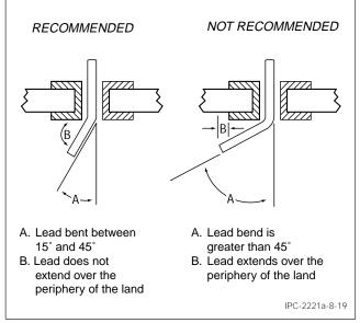
Figure 8-19 Partially Clinched Through-Hole Leads
