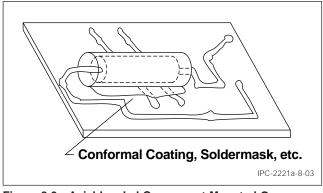
Figure 8-3 Axial-Leaded Component Mounted Over Conductors
