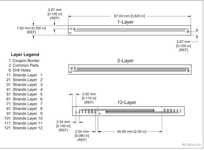
Figure 12-22 Test Coupon X, mm [in]
