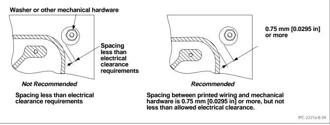
Figure 8-4 Uncoated Board Clearance
