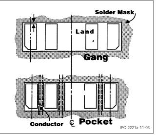
Figure 11-3 Solder Resist Windows
