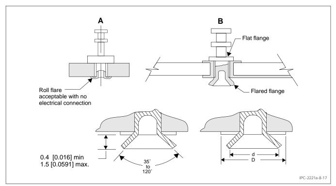
Figure 8-17 Standoff Terminal Mounting, mm [in]
