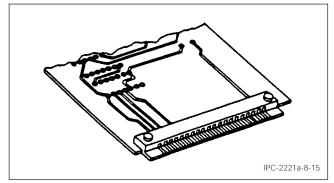
Figure 8-15 Edge-Board Adapter Connector
