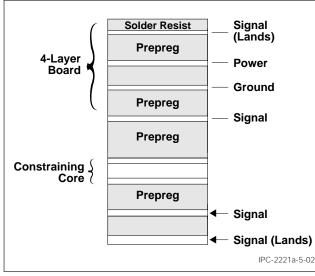
Figure 5-2 Typical Asymmetrical Constraining-Core Configuration
