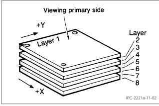
Figure 11-2 Multilayer Board Viewing
