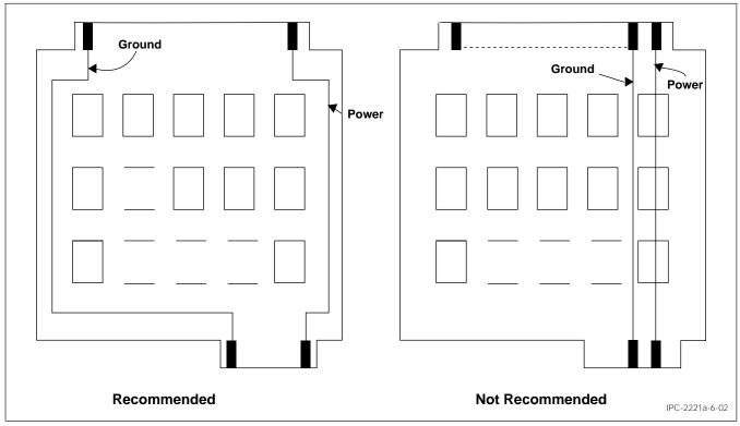
Figure 6-2 Single Reference Edge Routing
