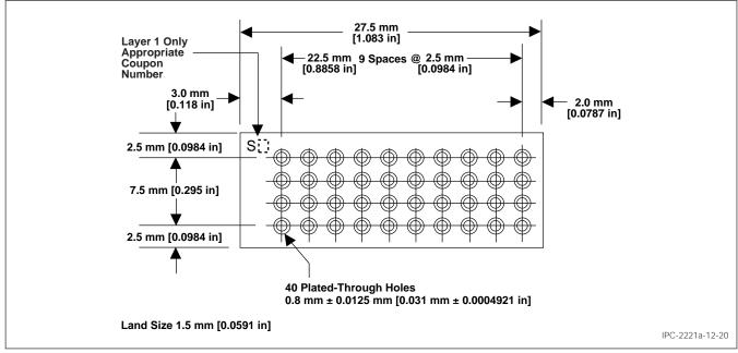
Figure 12-20 Test Coupon S, mm [in]
