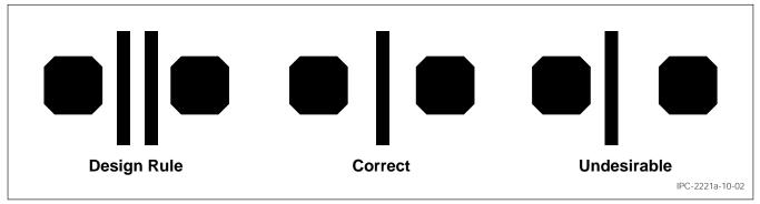
Figure 10-2 Conductor Optimization Between Lands
