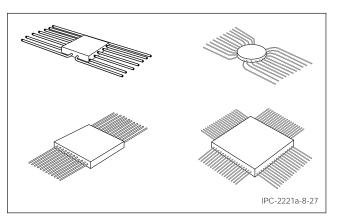
Figure 8-27 Flat-Packs and Quad Flat-Packs
