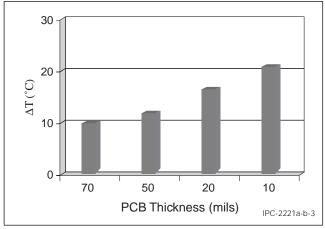
Figure B-3 Board Thickness
