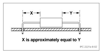
Figure 8-2 Component Body Centering
