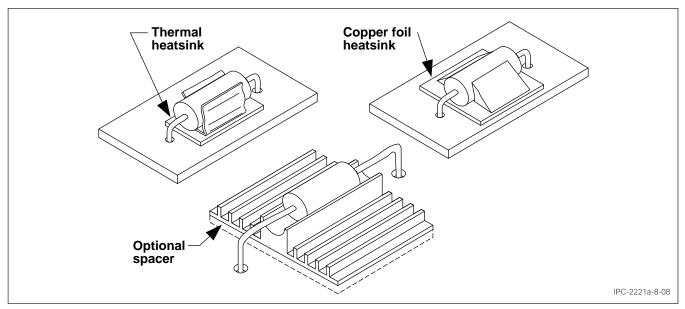
Figure 8-8 Heat Dissipation Examples
