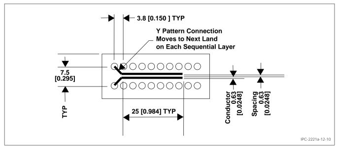
Figure 12-10 Coupon E, mm
