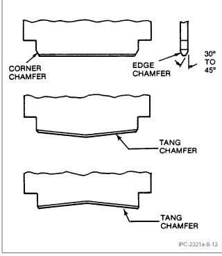
Figure 8-12 Lead-In Chamfer Configuration
