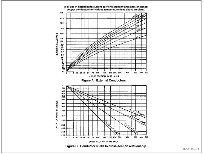
Figure B-2 IPC 2221A External Conductor Chart
