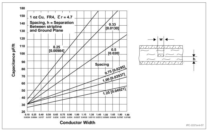
Figure 6-7 Capacitance vs. Conductor Width and Spacing for Striplines, mm [in]
