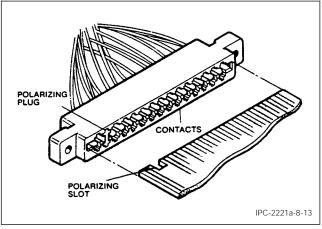
Figure 8-13 Typical Keying Arrangement
