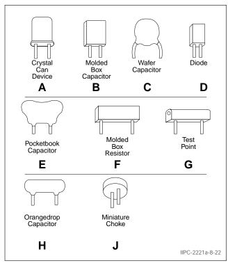
Figure 8-22 Two-Lead Radial-Leaded Components
