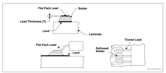
Figure 8-32 Examples of Flat-Pack Surface Mounting
