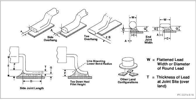
Figure 8-16 Round or Flattened (Coined) Lead Joint Description
