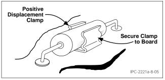
Figure 8-5 Clamp-Mounted Axial-Leaded Component
