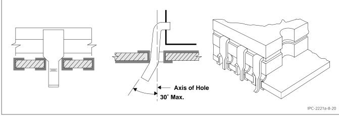
Figure 8-20 Dual In-Line Package (DIP) Lead Bends
