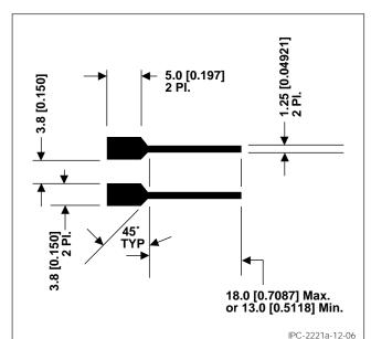
Figure 12-6 Coupon C, External Layers Only, mm [in]
