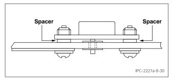
Figure 8-30 Metal Power Package with Resilient Spacers
