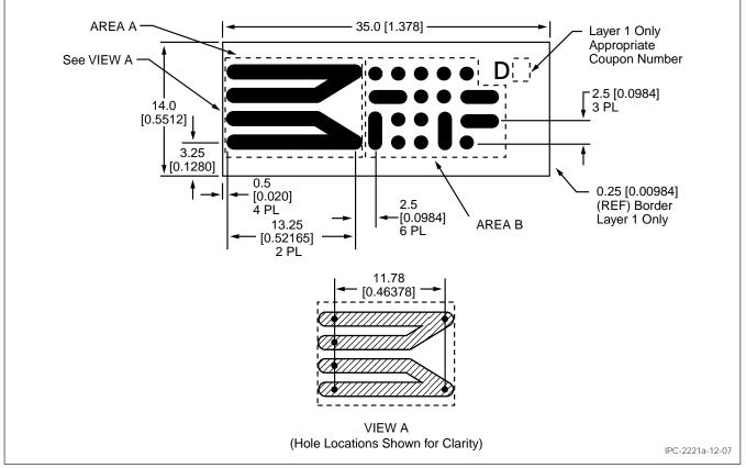
Figure 12-7 Test Coupon D, mm [in]
