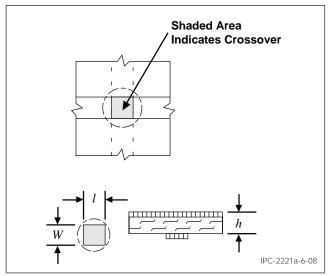
Figure 6-8 Single Conductor Crossover
