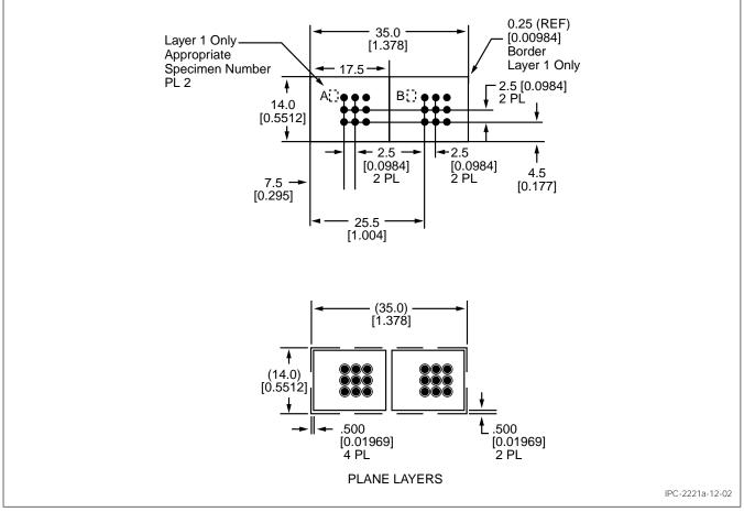
Figure 12-2 Test Coupons A and B, mm [in]
