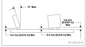
Figure 8-23 Radial Two-Lead Component Mounting, mm [in]
