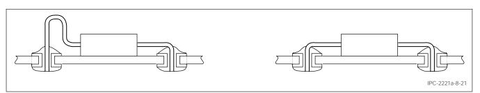
Figure 8-21 Solder in the Lead Bend Radius
