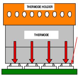
HEAT IS CONDUCTED FROM THE THER MODE TO THE PARTS AND SOLDER
