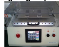
Sliding Test of FPC
