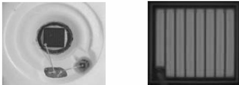
Fig. 1: Golden Dragon II LED. Left: Chip with bonding in its housing, right: close-up view of the irradiating surface and the bonding wire in the lower left corner. Emitting surface is 0.94 mm x 0.94 mm.
