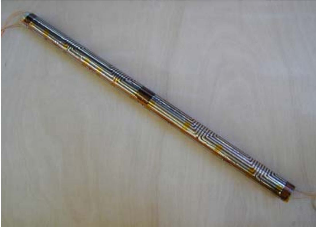
Picture 4: Polyimide foil heater without top layer mounted to a tube diameter 60 mm.
