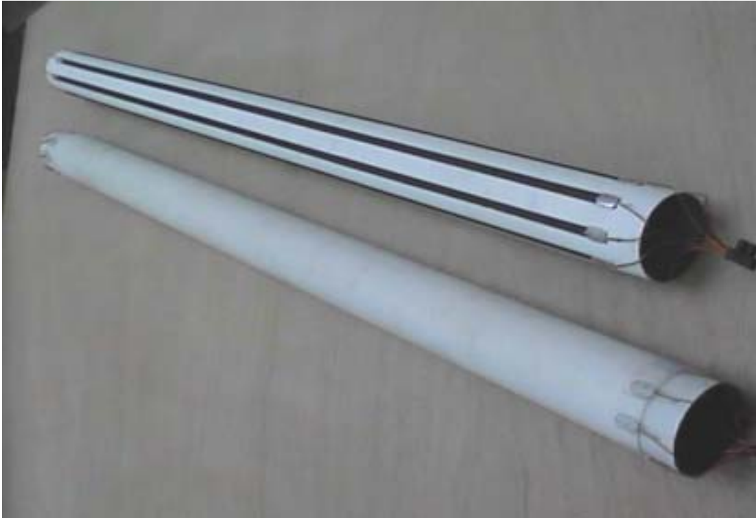
Picture 1: Tubes delivered by EMPA before (top) and after (bottom) top ceramic coating
