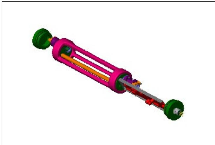
***Figure 2 – Cutaway view of new POC sensor.***
